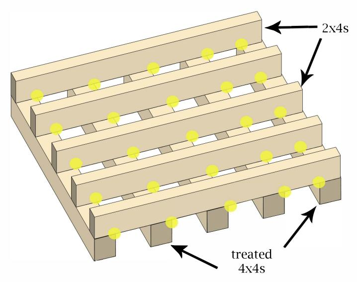
Use a metal truss hanger or strap at each intersecting point to securely attach the 2x4s to the 4x4s.
