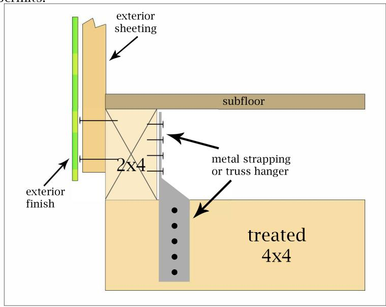
Take note that the exterior sheeting is NOT flush with the 2x4. When the forklift slides between the 4x4s and picks up the play-house by the 2x4s, the drag of the forks as they back away pulls the sheeting and exterior from the framing if flush.
